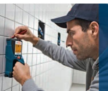
"It's definitely worth purchasing. Unlike our previous instrument, the D-tect 150 Professional can also find plastic pipes. The damage caused by drilling into one pipe costs more than the purchase price of the instrument."
